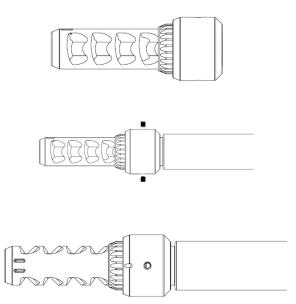
(4) To adjust your barrel tuner; shoot a three to five round control group with the tuner on the default setting (turn clockwise until it bottoms out, then counter clockwise until the witness mark on the tuner lines up with the closest adjustment mark on the locking collar and lock in place). Then starting in incriments of one, turn the tuner counter clockwise one adjustment mark, lock it down again and shoot two rounds.
